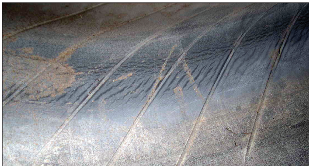
EFFECT: Inner Liner Marbling - Creasing CAUSE: Underinflation
