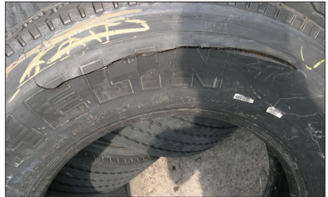
Fatigue Rupture or “Zipper”
