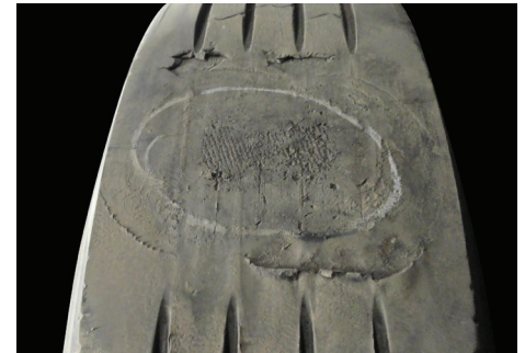
Brake Skid Damage
