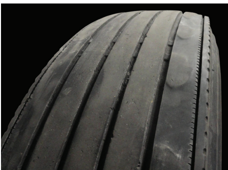
Depression Wear (Shoulder)
