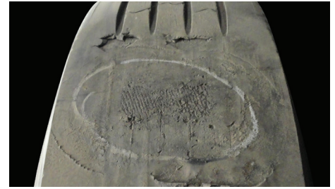
Brake Skid Damage
