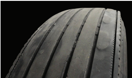
Depression Wear (Shoulder)
