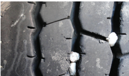
Stone Retention / Drilling
