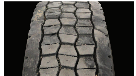
Cupping / Scallop / Alternate Lug Wear
