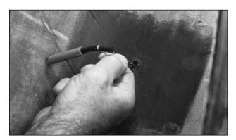
Remove spiral cement tool from the injury and feed the small end of the wire puller through the injury from inside of the tire.
