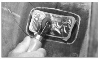
Stitch the repair unit, firmly pressing down from the center toward the outer edges. This will eliminate trapping air under the repair unit.
