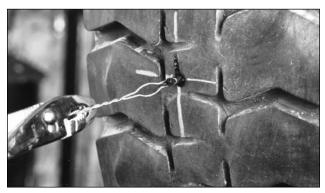
Grasp the wire puller from the outside of the tire and begin pulling the stem into place. If the wire puller comes off, grasp the stem with a pair of pliers and pull the stem until it fills the injury, exposing approximately 1/2 inch (13 mm) of the gray cushion bonding gum above the face of the tread.
