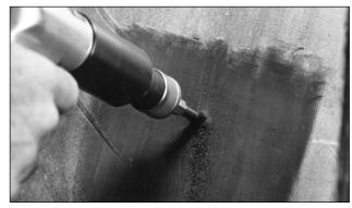
Prepare the injury with the proper size carbide cutter on a low rpm drill (max. 1200 rpm).
