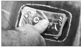
With the tire beads in a relaxed position, center the repair unit over the filled injury. Press the repair unit down into place over the injury. Make sure the directional bead arrows on the repair unit are aligned with the beads of the tire, and press into place. Roll the protective poly back to the outer edges of the repair unit. This enables you to handle the repair unit without contaminating the bonding gum layer. You are now ready to stitch the repair.
