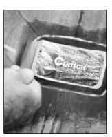
Remove the rest of the poly backing. Stitch the repair unit from the center to the outer edges. Remove the top clear protective poly.
