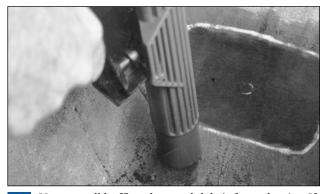
Vacuum all buffing dust and debris from the tire. If the buffed surface is touched or contaminated after cleaning the area, you must repeat Step 11 to guarantee your surface is clean for proper repair bonding.
