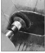
Use a low rpm (max. 5000 rpm) buffer and texturizing wheel to mechanically buff the stem flush to the inner liner. Then buff the outlined area to achieve an even RMA-1 or RMA-2 buffed texture. Use a clean, soft wire brush, remove all dust and debris from the buffed area.
