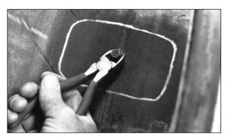
Remove the template and cut off the stem 1/8 inch (3 mm) above the inner liner on the inside of the tire. NOTE: If you do not have a repair template, go to this step and cut the stem; then using the correct sized patch and centering it correctly on the injury – arrows towards the beads – draw your perimeter approximately 1/2 inch larger than the repair patch.
