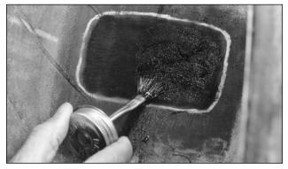
Using Chemical Vulcanizing Fluid (cement), brush a thin, even coat into the clean textured area. Allow 3 to 5 minutes to dry; the vulcanizing cement should be tacky. Areas with high humidity may require a longer dry time. Make sure the cement used is compatible with the repair units you are installing.
