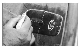
On the inside of the tire, center the appropriate repair unit template over the stem, make sure to correctly align the template in relationship to the tire beads, and draw a perimeter around the template.
