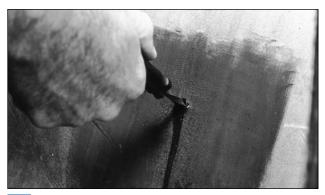
Using a Spiral Cement Tool, cement the injury from the inside of the tire with Chemical Vulcanizing Fluid. Turn the tool in a clockwise direction both into and out of the tire. This step should be repeated 3 to 5 times. Leave the tool in the injury as you go to the next step.
