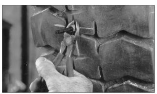
Cut the stem off on the outside of the tire 1/8 inch (3 mm) above the tire's surface. The tire is now ready to be returned to service.
