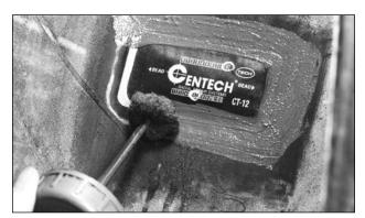
To cover over-buffed areas in tubeless tires, apply Security Sealer to the outer edge of the repair unit and over-buffed area. If tube-type, cover the repair with Tire Talc to prevent the repair from vulcanizing to the tube.
