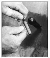
Place the wire puller in the middle of the black exposed portion of the stem. Remove the protective poly from the stem and brush a light coat of Chemical Vulcanizing Fluid (cement) on this area. For lubrication, apply a coat of cement to the wire puller where it contacts the stem.
