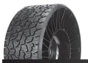
Airless Radial tire designed for zero-turn and stand-on mowers.
