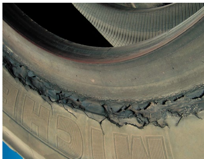
Damage on the bead due to overloading of the vehicle
