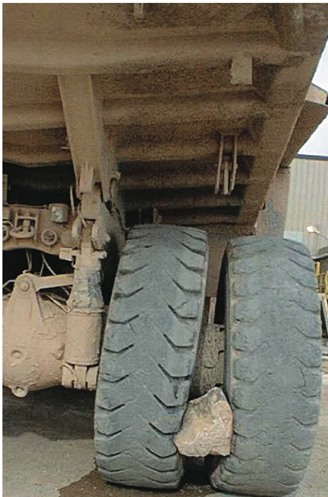
Beware of stones being ejected when demounting dual tires!
