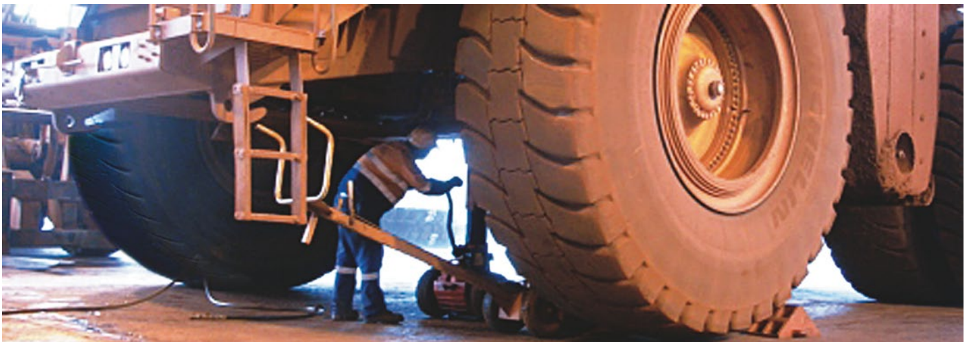
To adjust the suspension, the vehicle must be placed on blocks
