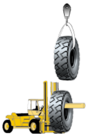
Holding the tire too tightly may distort it
