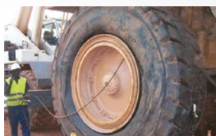
13 Inflate to mounting pressure, then adjust to working pressure
