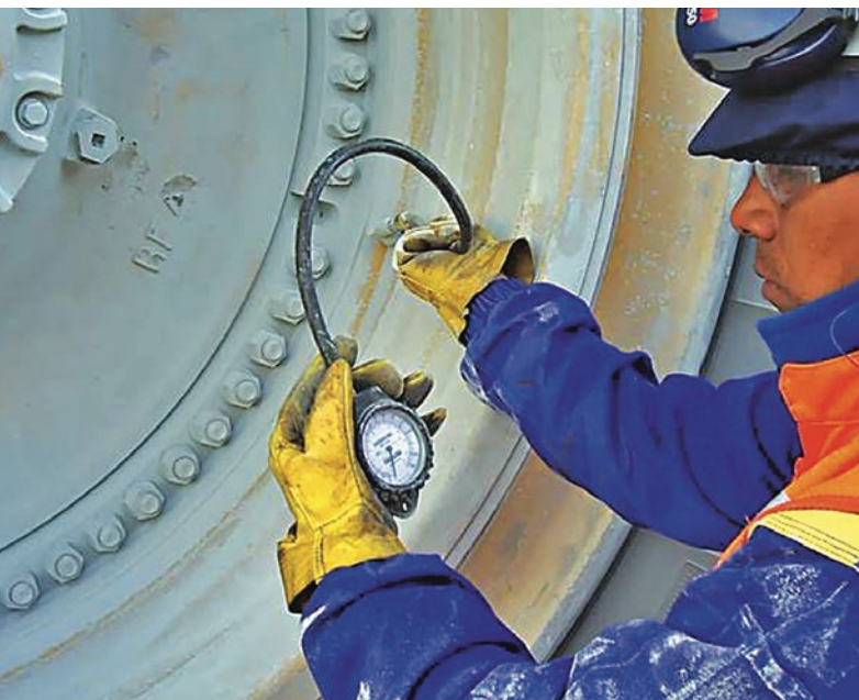
Keep to the recommended inflation pressure
