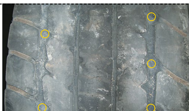
MICHELIN® X-CRANE® with the bridges on the shoulders and the lengthwise grooves in the center regrooved (bridges in the center and outer lengthwise grooves not regrooved)
