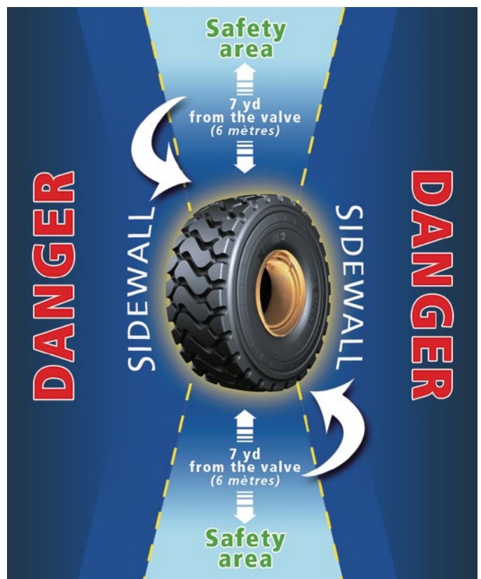
Always stand facing the tread during inflation
