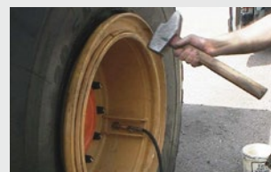
12 Inflate and lightly tap the locking ring
