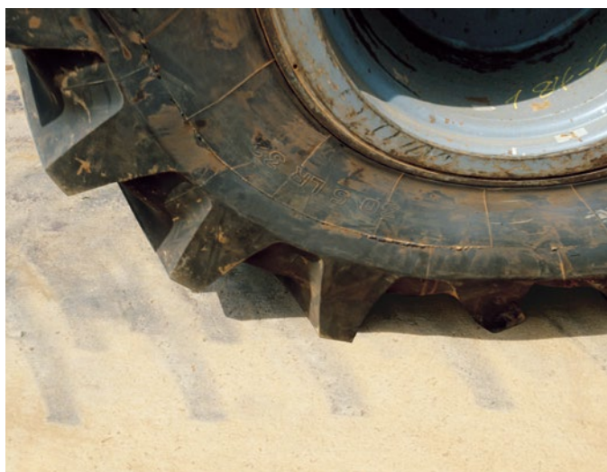
Underinflation adversely affects the service life of the tire
