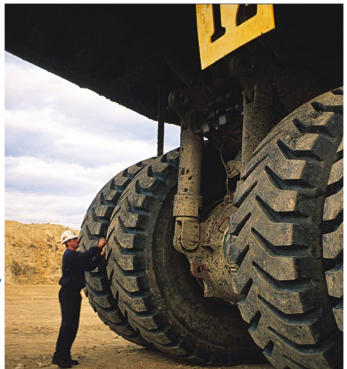
Check there are no objects trapped between the tires of a dual tire unit
