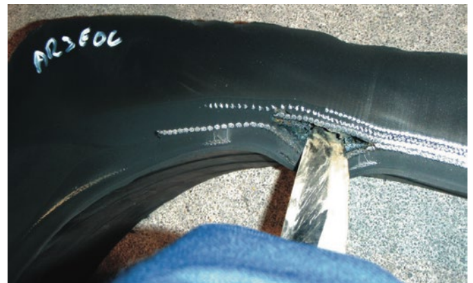
Separation of the components in a tire
