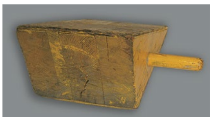
A wooden wedge left inside a tire during mounting...
